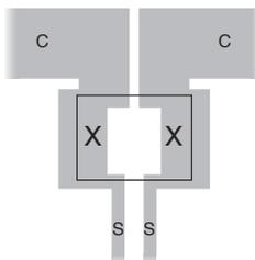
Note: Actual width of current trace is based on magnitude of current. Point of connection should be in the area shown.
